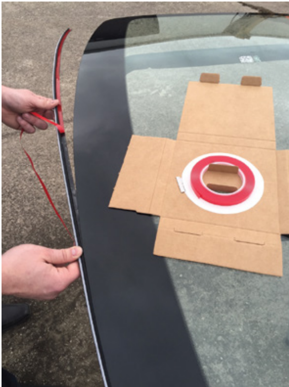
Re-Attaching Retainer on FW3091
