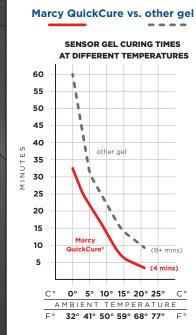
\*To replicate the most demanding conditions, Marcy QuickCure gel was dispensed only after it reached ambient temperature. Quicker cure times can be achieved, even in sub-freezing temperatures, by keeping the gel at room temperatures prior to dispensing.
